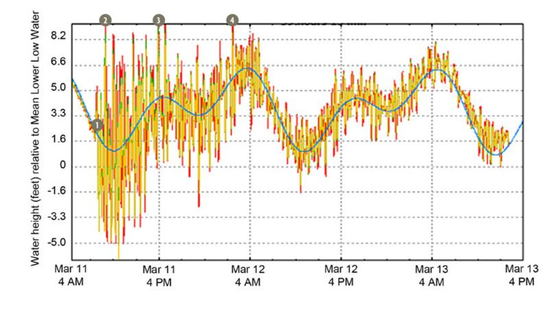
Water level recording from the Grescent City Tide gauge during the Japan tsunami. The blue line is the tidal fluctuation and the yellow/red line shows the actual water height relative to the average low tide height.
