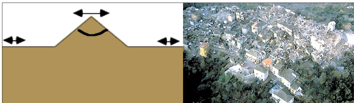
Figure 13. Hilltop amplification is the result of the seismic wave energy being concentrated at the top of a hill. Left: If the ground were flat, the ground shaking is some uniform value as represented by the arrows to the left and right of the hill. The hilltop concentrates the seismic energy, resulting in much strong shaking (represented by the longer arrow at the top of the hill). Irpinia, Italy felt the effects of hilltop amplification in the 1980 M 6.9 earthquake. Notice how the damage is concentrated near the peak of the hill.
