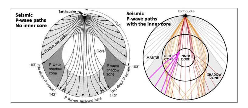
An illustration of how seismic waves are bent by interfaces within the earth - on the left, no inner core, on the right, with an inner core. The purple paths show the arrivals that Lehmann observed. Note - the illustrations are simplified and not to true scale.
